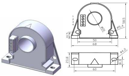
definition of connection end End 1: power supply anode End 2: power supply cathode End 3: output of signal anode End 4: input of signal cathode
