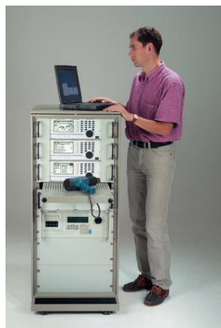
3-phase version of the SYS61K with 3 x LMG95 power measuring device and source 3 x 5 kVA
