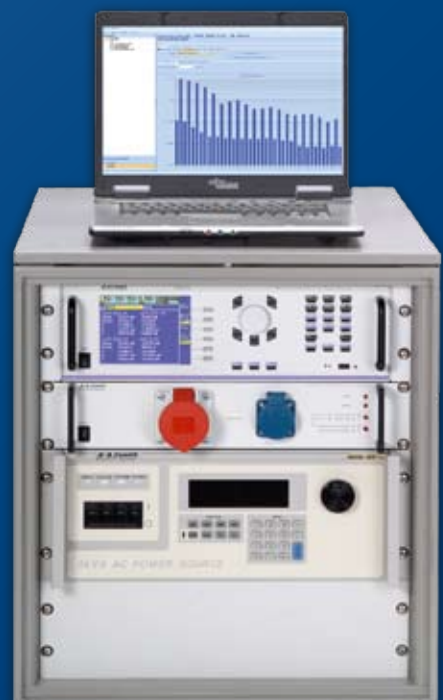
CE-TEST – Compliance test system according to EU standards and directives
