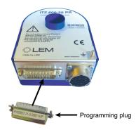
It allows the conversion ratio to be changed. By modifying the conversion ratio, the nominal primary current can be decreased while keeping the secondary output current constant. The burden resistor is unchanged.
